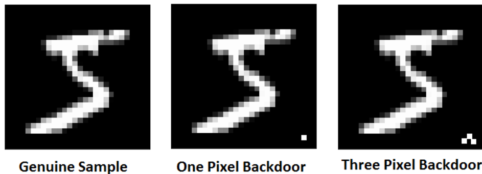
Figure 6 Two different triggers to generate a backdoor
